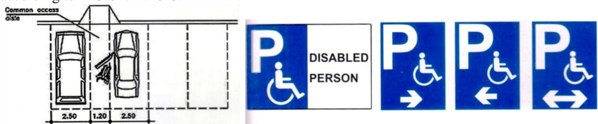
Parking requirements and signage for specially abled person's parking (Image source: IRC: SP: 12-2015)
